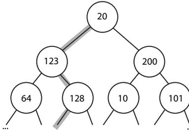
Now imagine a CUDA program where each CUDA thread computes the sum of results obtained by applying the functions  $f()$  or  $g()$  to all numbers on a path from the root to a leaf. The path taken through the tree is determined by the thread's id, as given in the code below. (In the figure above we highlight the path for thread id 2 which in binary is ...00000010 or left-right-left-left-left...)
