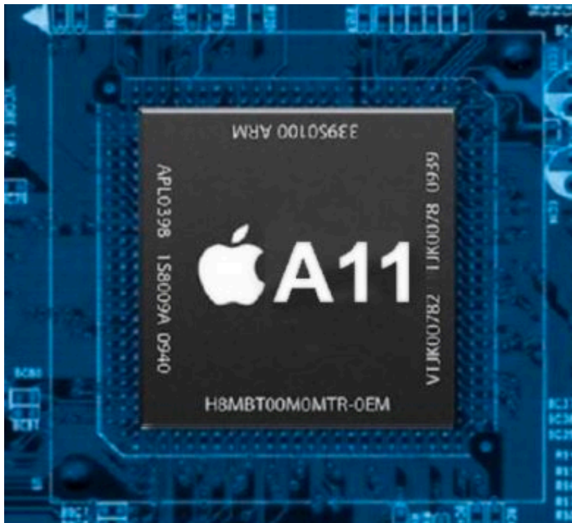
Apple A11 Heterogeneous SoC multi-core CPU + multi-core GPU + media ASICs + AI basics
