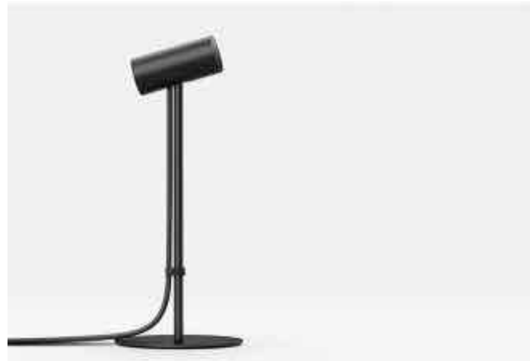
60Hz IR Camera (measures absolute position of headset 60 times a second)
