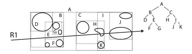
B. One of the nice properties of a bounding volume hierarchy (BVH) is that it can be efficiently updated ("refit") when a single primitive contained in the hierarchy is moved. Refitting modifies the BVH so that the BVH property is maintained: *the bounding box of a node is a bound containing the primitives in all child nodes*. Refitting does not modify the structure of the BVH – **it only updates bounding boxes for some of the tree's nodes based on the new bounds of leaf nodes**.
