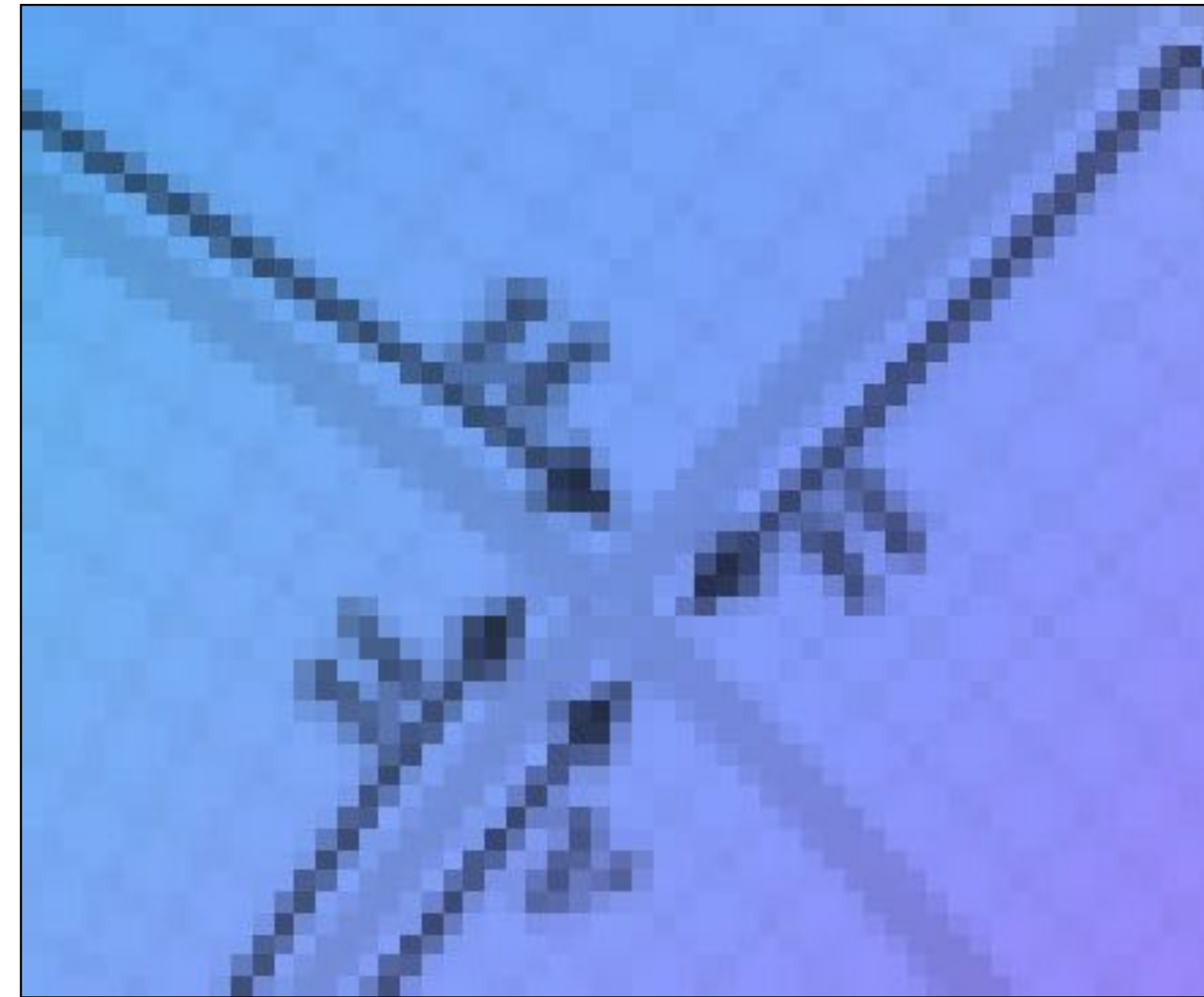
Pre-filtered texture map (high frequencies removed)
